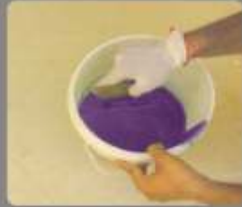
Slowly add the required amount of powder filler & mix to creamy consistency
