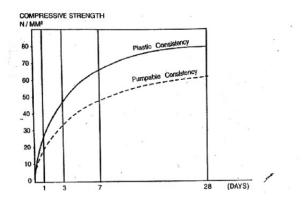
Compressive strength of CEMGROUT - NS (GP-2) in plastic and pumpable consistencies @ standard lab conditions.
